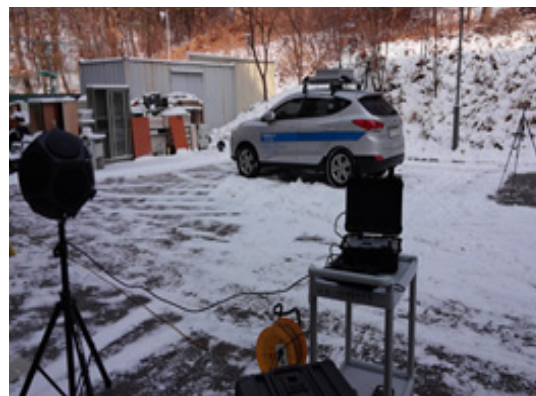
Fig. 3. Pink Noise Measurements in Research Institute of Public Health and Environment with noise mobile monitoring vehicle and portable sound level meters.
