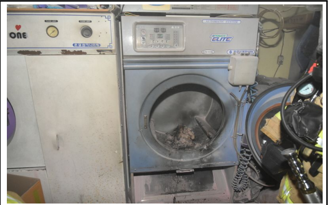
Fig. 2 laundry dryer inside (Only the clothes, etc. have soot on the laundry dryer)
