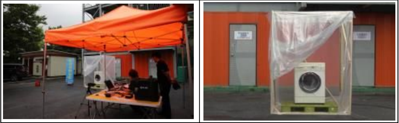
Fig. 8. The scene where the vapor occurs in the dry laundry by using the organic solvent within drier 4 | 1192 지휘대119!
