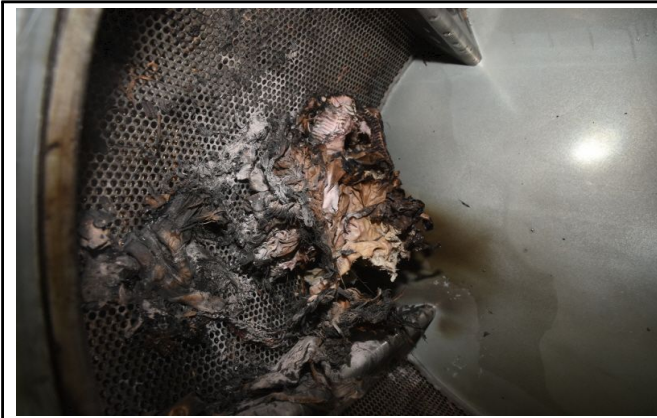
Fig. 1 laundry dryer carbide (Fire limited to the inside of the laundry dryer of the initial ignition unit)
