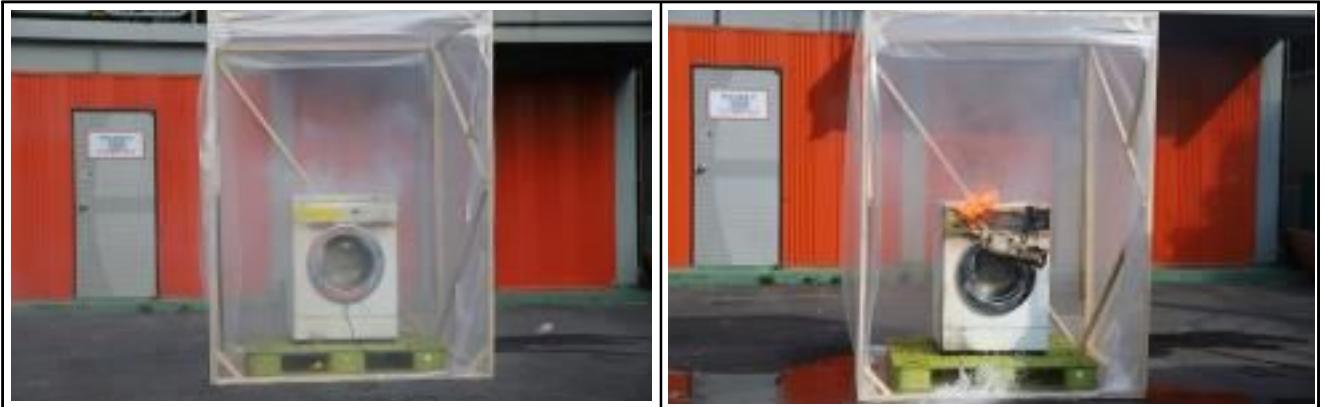
Fig. 10. The scene where the vapor occurs in the dry laundry by using the organic solvent within drier
