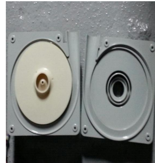
흡입팬 Overhaul 후
