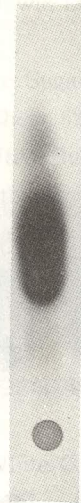
Fig. 2. Thin-layer chromatogram of HIGH FRUCTOSE CORN SYRUP in Standard Oriental bee honey by Charcoal Column.
