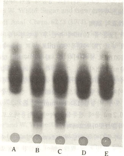
Fig. 4. Thin-layer chromatogram of HIGH FRUCTOSE CORN SYRUP in Pure marketing Honey and Standard HFCS. A. Acacia Honey B. 42%-HFCS (M. co) C. 55%-HFCS (M. co) D. Rape Honey E. Wild Honey
