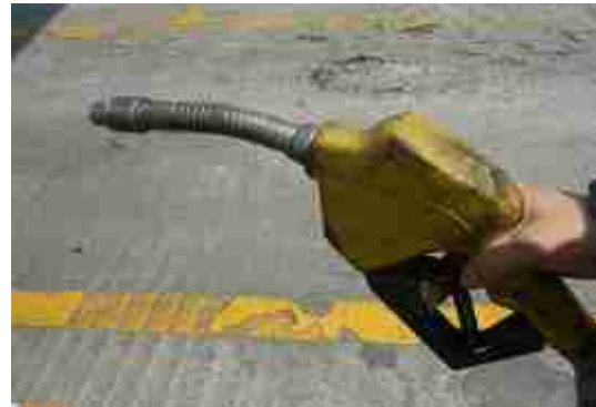
Fig 5. Refueling system whithout VOCs recovery system.
