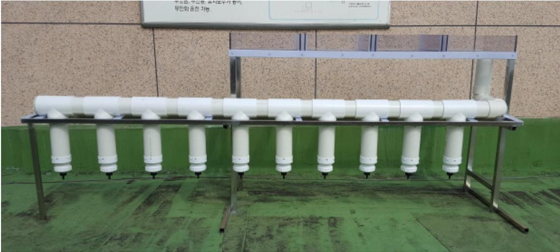
**Fig. 1.** Stepwise rainwater collecting sampler on the roof of a four-story building in seoul.
