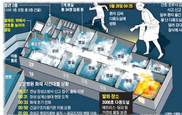
Figure 4. the Jang-Seong Nursing Hospital (JSNH) fire in 2 nd floor.
