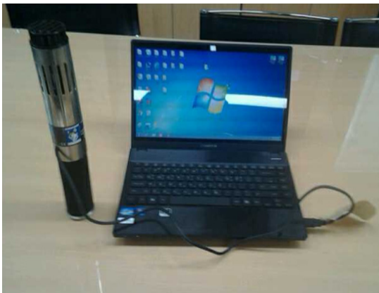
Fig. 3. TVOCs monitoring system using PID sensor.
